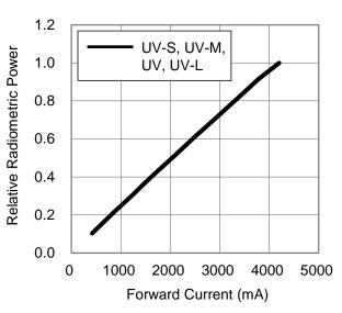
Fig 2. Relative Radiometric Power vs. Forward Current for UV-S, UV-M at T<sub>J</sub>=25 maintained.
