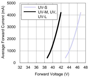
Fig 1. Forward Current vs. Forward Voltage for UV-S, UV-M.
