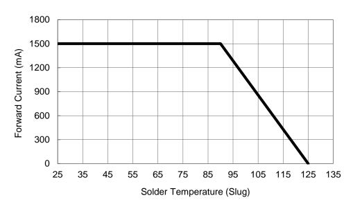
2. UV-M, UV, UV-L  $(T_{JMAX} = 125^{\circ}C)$
